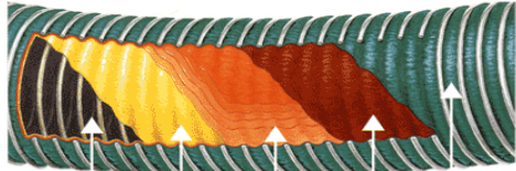
Inner Helix Polypropylene Inner Fabric and Films Vapor Barrier Films Reinforcing Fabric PVC-impregnated Nylon Cover and Outer Helix
